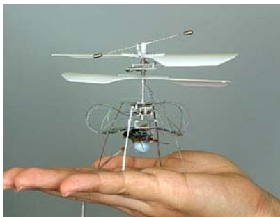
Figure 6. Micro flying robot which uses an piezoelectric motor (by Seiko Epson Corporation), reproduced from [6].
