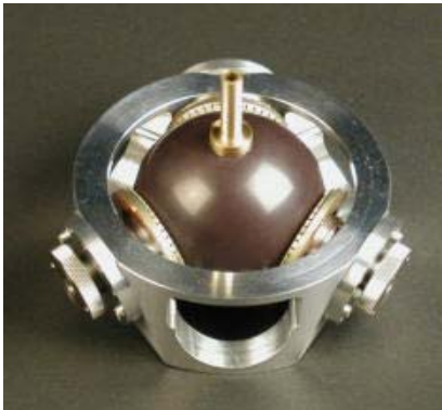
Figure 5. Spherical piezoelectric motor, made in Toyama Laboratory, Japan, reproduced from [5].
