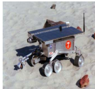
Figure 4. The robot Rocky 7 with USMs, used in planetary exploration environments, reproduced from [4].
